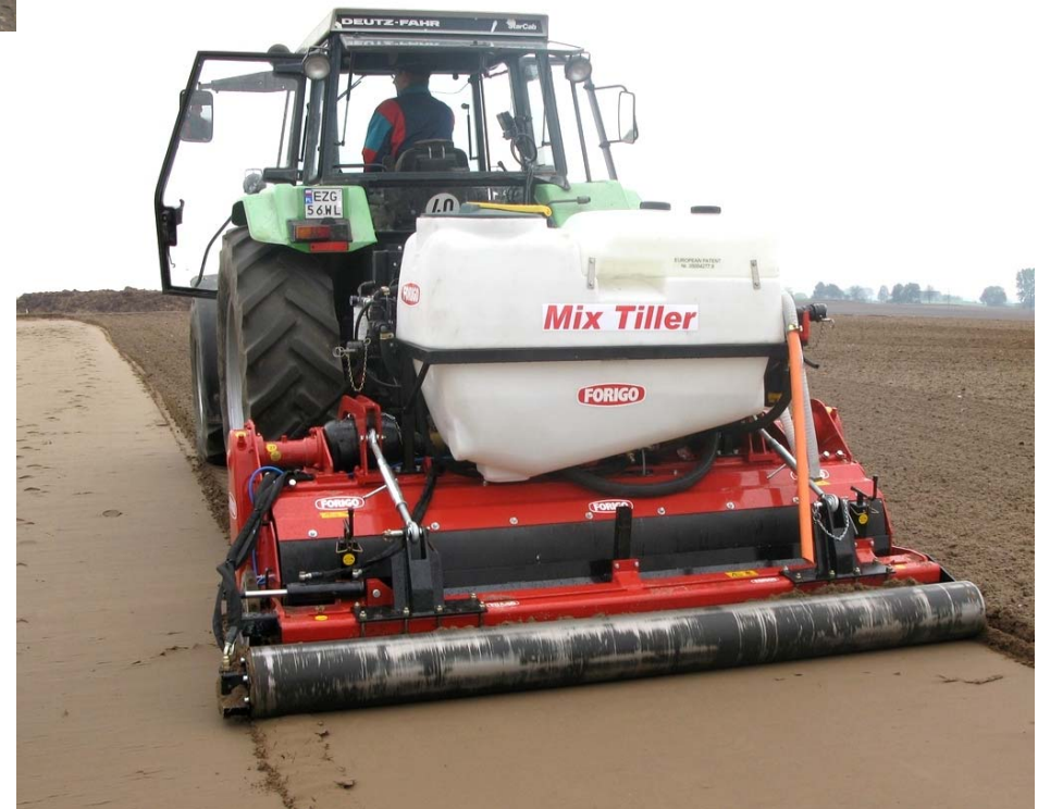
A compact metam sodium applicator of 2.5 m working width, suitable for greenhouse and field applications
