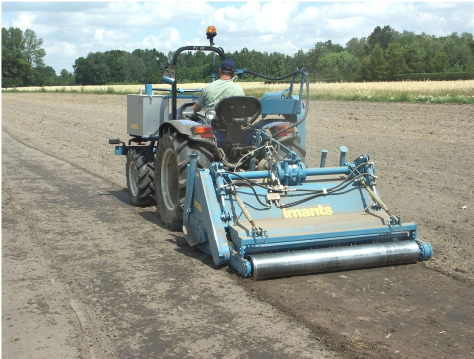
A tractor-mounted metam sodium applicator of 1.5 m working width, used for soil treatment in greenhouses
